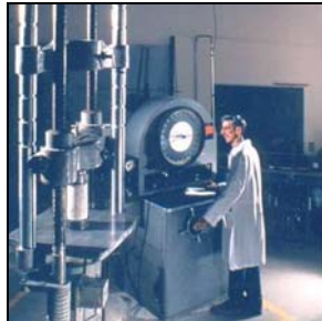
Baldwin BTE 120 Universal Test Machine Richmond Laboratory
