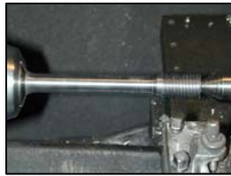
Machining of Tensile Test Specimen
