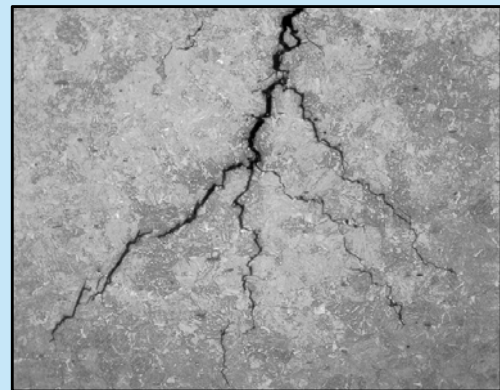
Stress corrosion cracking of carbon steel that preceded catastrophic failure. Magnification approximately 67 X.
