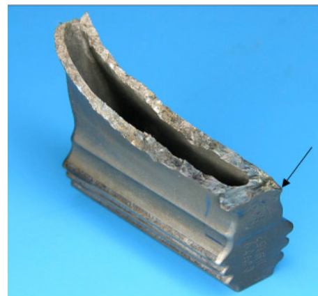
Blade failure by high cycle fatigue; arrow indicates origin
