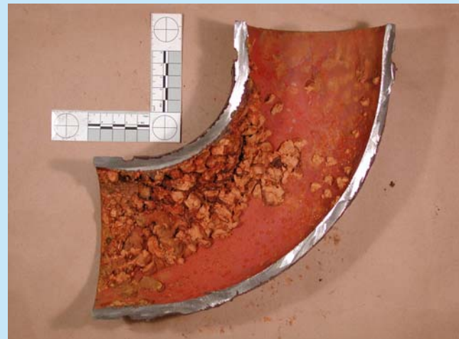
Tubercule formation due to microbiological activity observed on the internal diameter surface of a ductile iron fitting.
